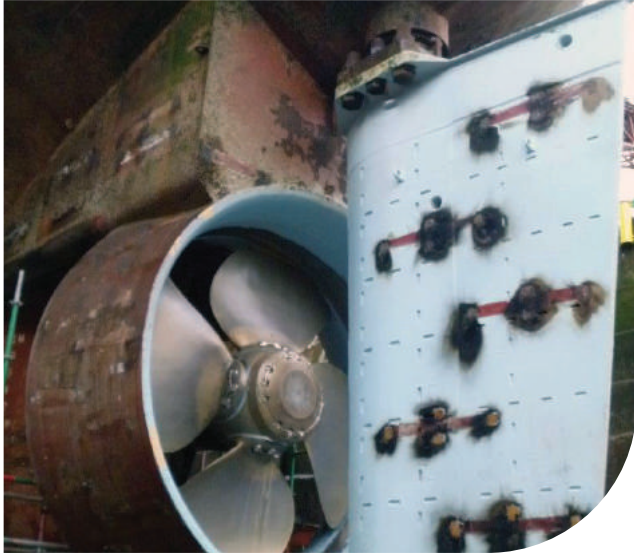
Rudder and Kort Nozzle in perfect condition after 18 months in-service
